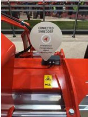
'Connected shredder' is an application for mobile phones with Android / IOS systems, which can monitor the real-time basic parameters of the shredder. The main objective is to ensure triggering of alarms in case of exceeding the threshold speed of the rotor, the oil temperature, rotor vibration, and to recommend routine or extraordinary maintenance based on the overall condition of the machine. This solution contributes to a significant reduction in operating costs and eliminates downtime.
