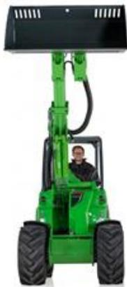
Avant 860i is one of the two largest and most powerful models of versatile telescopic loaders produced by Avant Tecno Oy. Nearly 2 tons of load-bearing capacity and 3.5-meter range make AVANT 800 the most distinctive compact loader among models available in the market. Machines of AVANT 800 series weigh 2.5 tons and have a width of 1.5 m, length of 3.4 m and height of 2.2 m. The articulated design combined with modern design guarantees the highest level of mobility.
