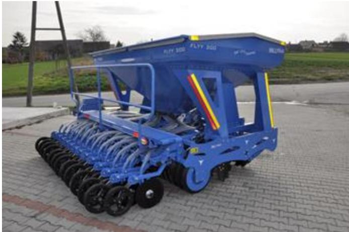
Namyslo FLYY - wide feeding hopper- disc sowing - direct seeding into stubble - double disc coulters - GPS System - ISO BUS connection
